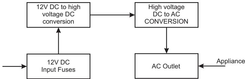
The DC to DC converter stage uses modern high frequency power conversion techniques that have replaced bulky transformers found in less technologically advanced models. The inverter uses advanced MOSFET transistors in a full bridge configuration, which ensures excellent overload capabilities and allows the inverter to operate reactive loads such as small induction motors.
